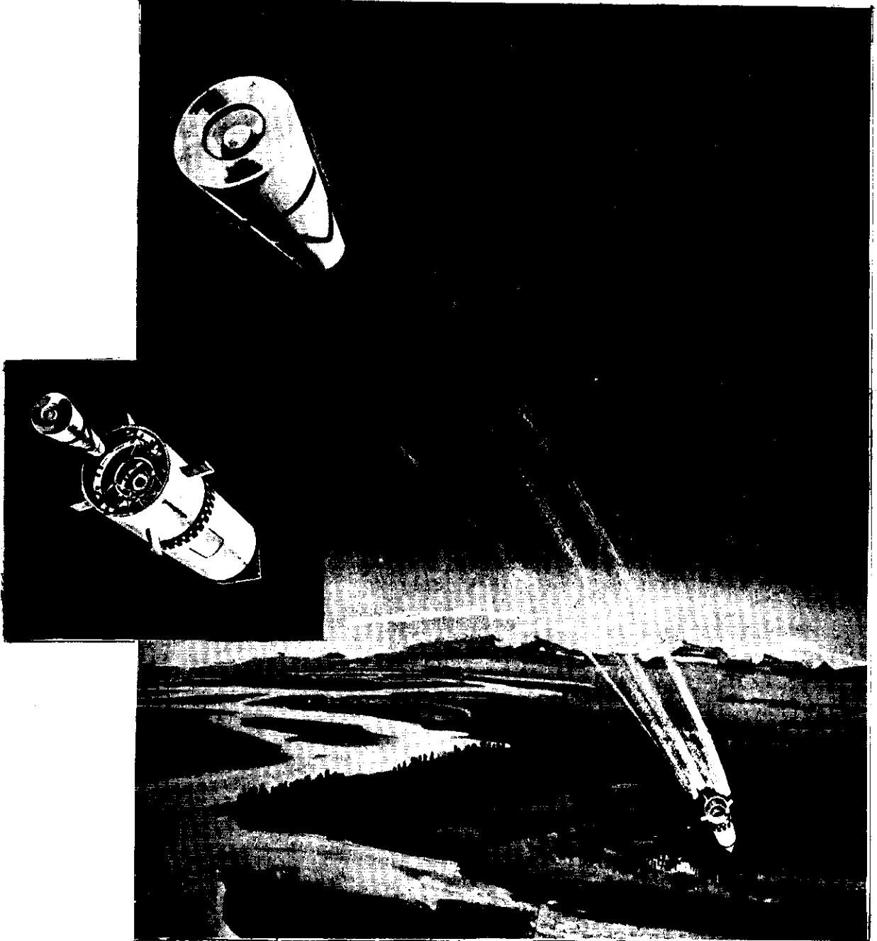
Television Capsule. After ejecting from the Redstone Tactical Body (inset), the capsule lags behind transmitting pictures of the terrain.
